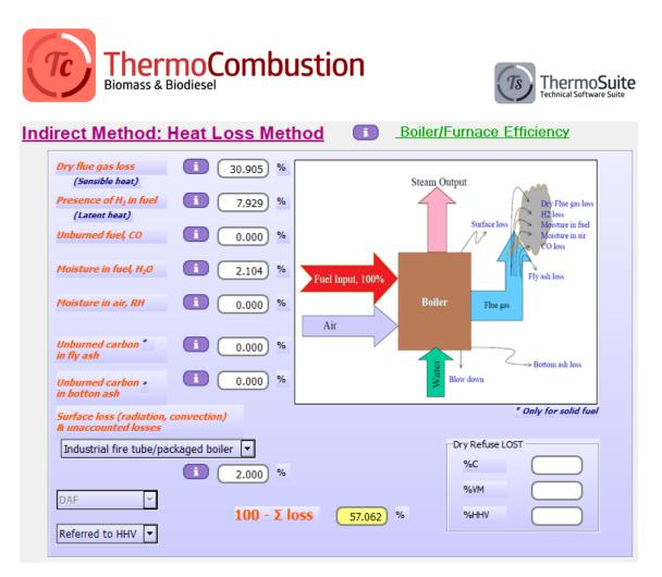
There is a higher efficiency (indirect method), because there is no loss due to unburnt.
